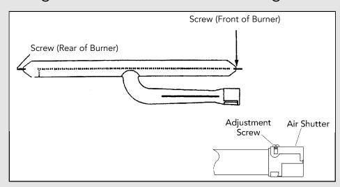
Remove screws securing glow bar igniter to burner box and place glow bar igniter aside. Remove screws securing metal plate to burner box located underneath griddle burner and remove metal plate.
